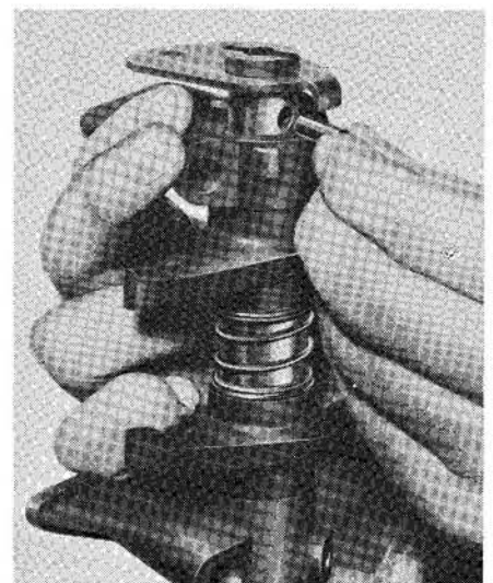
Fig. 21— To disassemble rocker arm assembly, set rocker arm on end and push front support down to allow removal of pin.
